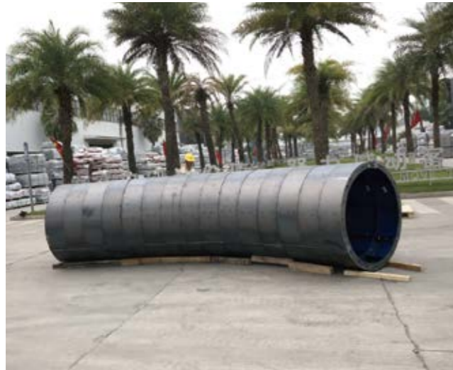
Steel Formwork for Circle Tunnel 圓形隧道鋼模板
